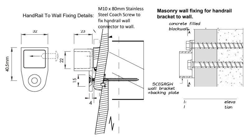
If Wall is a flat surface then mount with the above fixing directly onto the wall.
