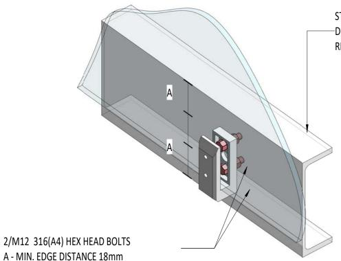
SEPARATION BETWEEN BOLT HEAD AND GLASS TO BE MAINTAINED.
