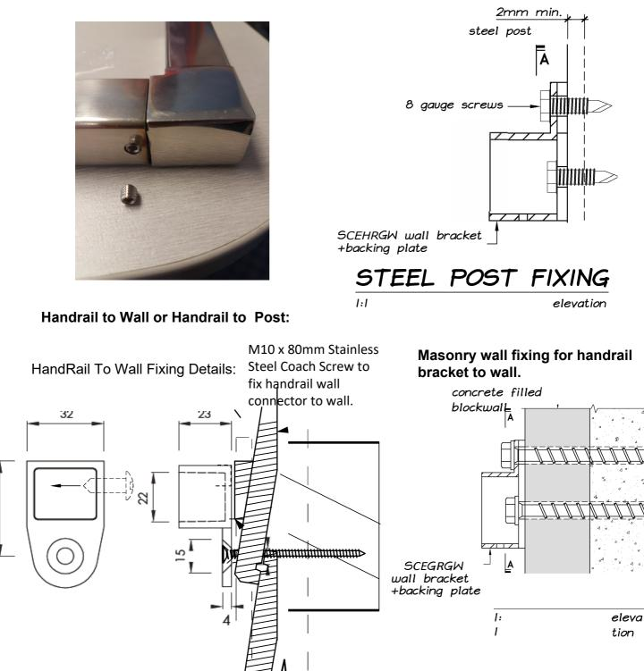
If Wall is a flat surface then mount with the above fixing directly onto the wall.
